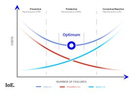
Figure 3 - *Relationship between maintenance costs and numbers of failures under different maintenance methodologies.*
